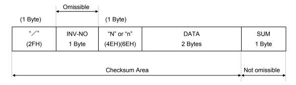
"N" or "n" (1 byte) : Communication error command. Also for check during an inverter trip (includes standing
