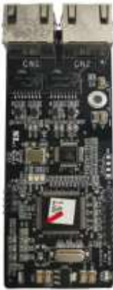
Ethernet/IP communication card EC-TX510/ EC-TX515
