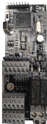
Programmable expansion card EC-PC502-00
