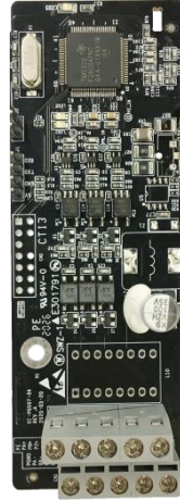
24V simplified incremental PG card EC-PG507-24
