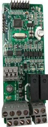
IO expansion card 2 EC-IO502-00
