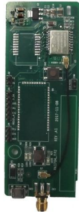
Bluetooth/WIFI communication card EC-TX501/502
