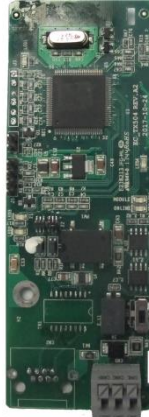
CANopen/CAN master/slave control communication card EC-TX505/511
