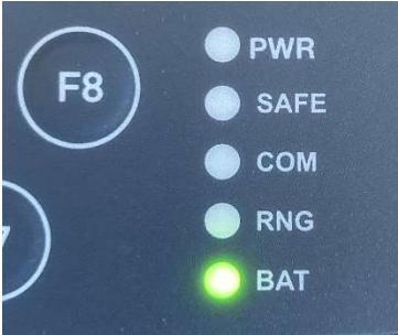
Illustration: Battery charge indicator light
