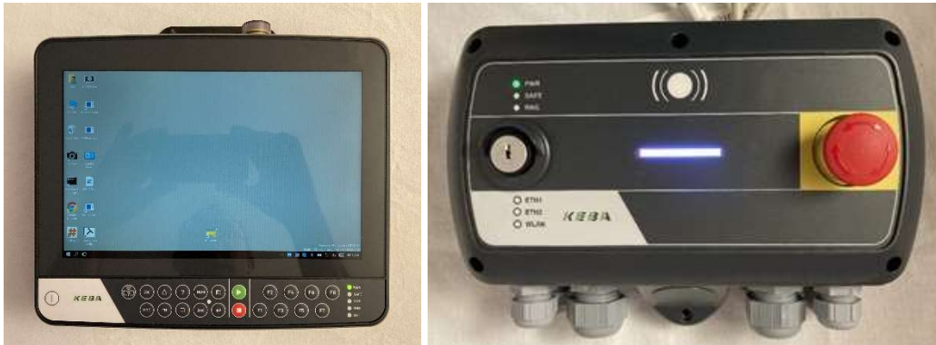
Illustration: Base station and handheld terminal
