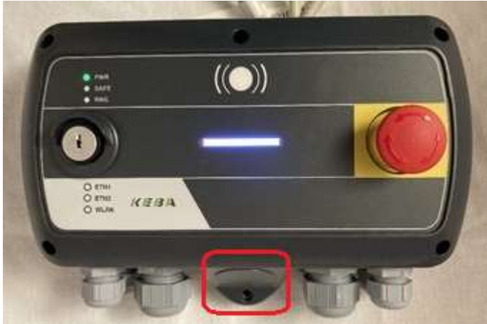
Illustration: Position of the pairing reset button
