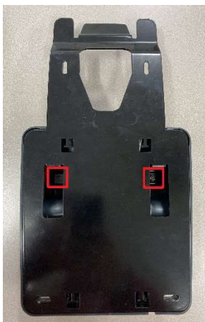
Illustration: Rear of the charging station with the marked screws
