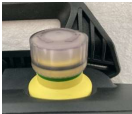
Illustration: Emergency stop not illuminated
