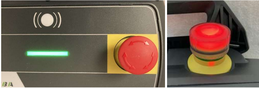
Illustration: Successful establishment of the connection between base station and handheld terminal
