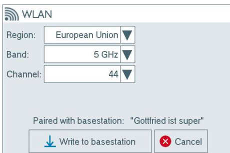
Illustration: Parameterization of the WLAN connection between base station and handheld terminal
