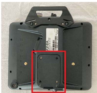
Illustration: Rear side of the handheld terminal with marked cover of the battery compartment
