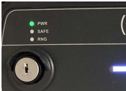
Illustration: PWR Led indicates power supply to the base station
