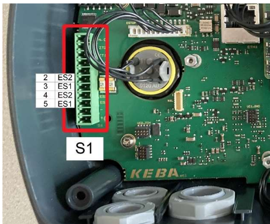
Illustration: Picture of the base station with terminal strip S1 - contacts for emergency stop (Pin 6 to 9)
