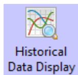
Historical Data Display component read data from specified HMI or PLC continuous registers periodically, and display them in grid.
