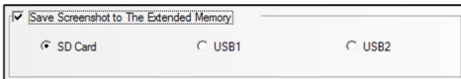
The bmp pictures are named as year-month-day, hour: minute: second: millisecond, for example: 2010-09-01, 10:12:50:203.bmp. User also can define the picture name by system special register. The LW9470~LW9485 define the prefix of file name, for example the constant in LW9470~LW9485 is "Version Num .20100001-" , then the screenshot picture name is Version Num .20100001-2010-09-01,10:15:28:421.bmp.
