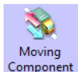
The Moving Component can change the display state and position according to the value of HMI register or PLC register.
