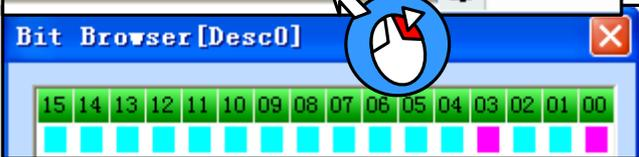
[Examples] For example RW9 value is 9, bit browser form RW9: 03,00 bit address can be seen in red: ON, decimal 9 to binary form as 0000 0000 0000 1001.
