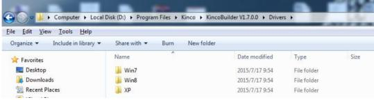
When connecting programming cable to MK series and PC first time, Windows system will detect new hardware and mention installing driver, users can install the driver according to the version of Windows.
